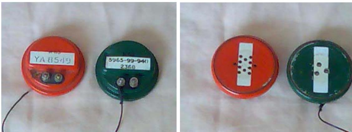
These inserts can be positively identified by measuring the DC resistance which will be 42 ohms at around 20 degrees C.
